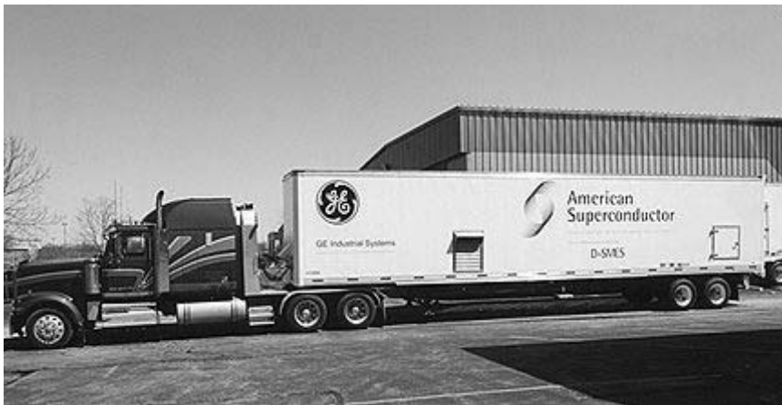
Figure 1 A trailer mounted D-SMES unit with 3MW and 16 MVA capacities (Picture supplied by American Superconductor)
